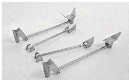
UNIVERSAL TRIANGULATED 4 BAR KIT 06-1509 - PLAIN STEEL 06-1509C - CHROME 06-1509S - POLISHED STAINLESS STEEL
